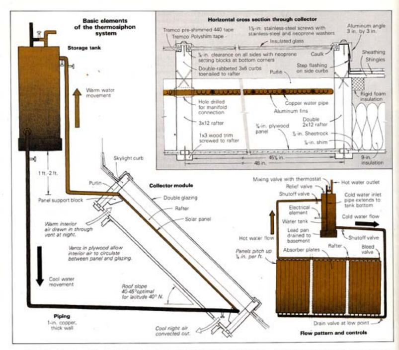
a result of settling will not occur. Once the tape is in place, we position two neoprene setting blocks (¾ in. by ½ in. by 4 in.) one-fourth of the way in from the bottom corners of the skylight rabbet to hold the glass panel ¾ in. away from the bottom edge.
